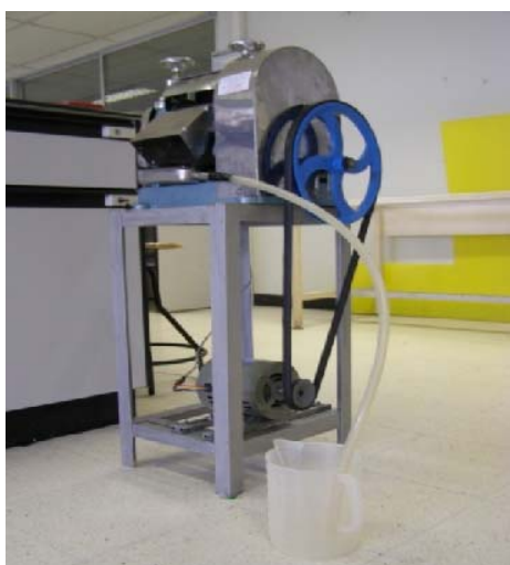
Fig. 1 sugar cane pressing machine with rolling press cylinders
