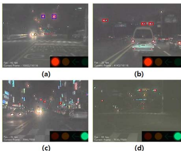
Fig. 7 (a) and (b) show red traffic light detection of red circle type and type of red circle and green arrow (c) and (d) show green traffic light detection of green circle type and type of green circle and green arrow
