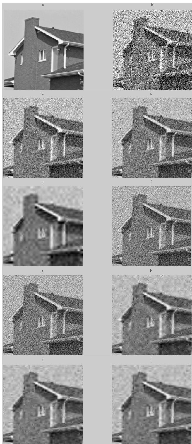
Fig 2,3 a) Original image. b) Gaussian noise with variance 0.06 is added to original image. c) Image denoising with median filter. d) Image denoising with wiener filter. e) Image denoising with global thresholding. f) Image denoising with stationary wavelet transform with hard threshold. g) Image denoising with stationary wavelet transform with soft threshold. h) Image denoising with Normal Shrink. i) Image denoising with Bayes Shrink. j) Image denoising with Modified Bayes Shrink (noisy pepper & noisy house)
