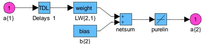
Fig. 11 Simulink Block Diagram of the layer2 of earth station NNC
