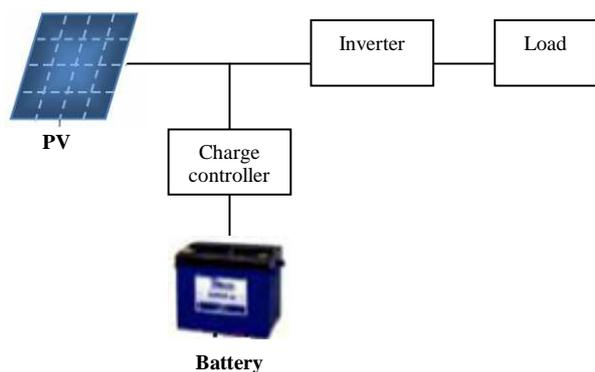
Fig. 1 Earth station power system architecture
