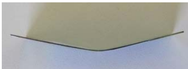
Fig. 6 Silicon foil shaped with a pressing mold of radius 10 mm
