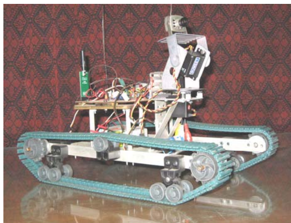
Fig. 4 The complete robot unit with the pan-and-tilt mechanism for better navigation
