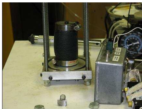
Fig. 4 Rubber bladder used to contain the propellant
