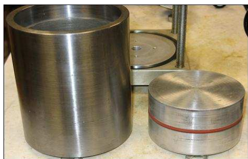
Fig. 5 The containment cylinder (left) and the piston (right) which fit inside the containment cylinder and used to separate the propellant from the pressurizing fluid
