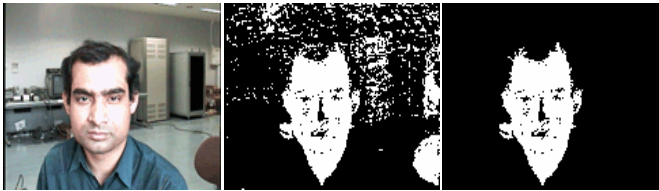
(a) Original image (b) Skin color segmented (c) Face area detected Fig. 4 Skin color segmentation
