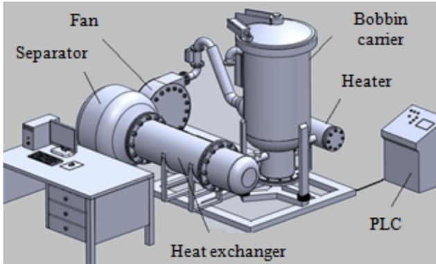
Fig. 1 General view of the experimental bobbin dryer
