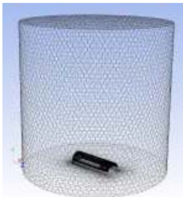
Fig. 8 Main geometrical features of the adopted grid inside the cylindrical sub-domain enclosing the building structure
