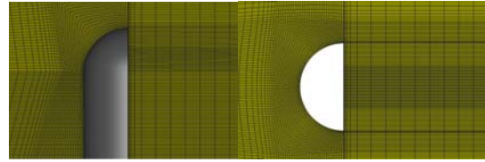
Fig. 3 Two views of the mesh in the vicinity of the SVM
