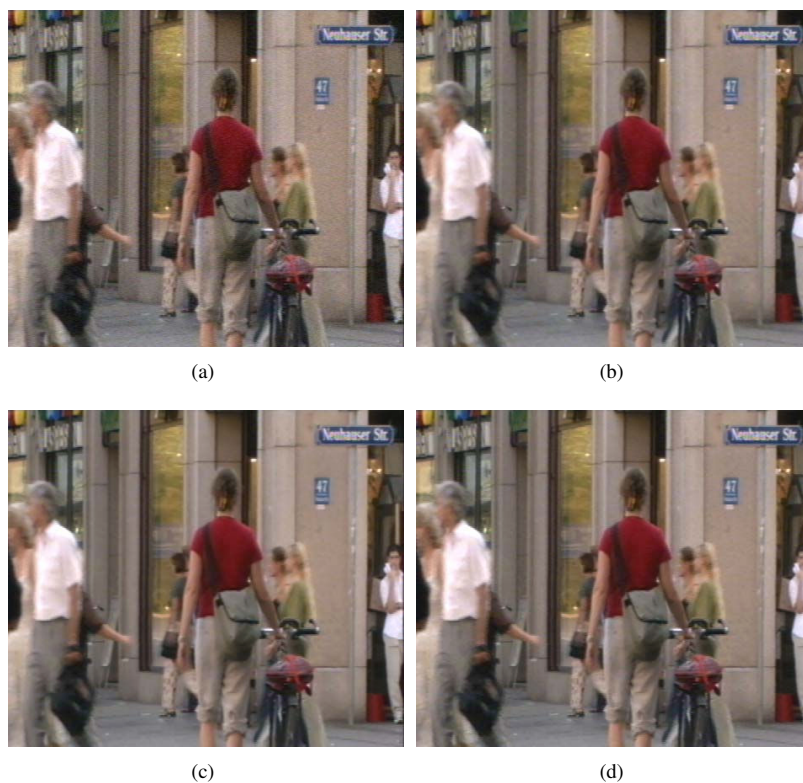
Fig. 8. (a) A frame from a real video sequence. (b), the result of the filtered frame with the two dimensional steering kernel, (c) the time symmetric kernel and (d) time asymmetric kernel.
