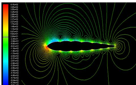
Fig. 13 static pressure distribution of NACA0012 airfoil and inflatable wing
