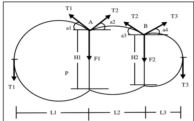
Fig. 6 stress analysis for inflatable wing
