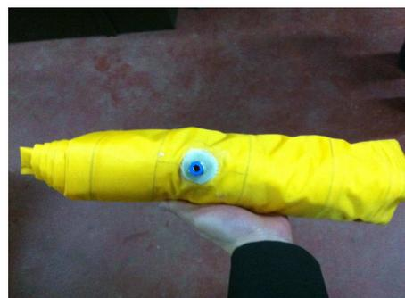
Fig. 15 heat sealing of the gas nozzle
