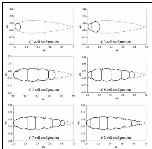
Fig. 5 internally tangential circular arc approach the airfoil
