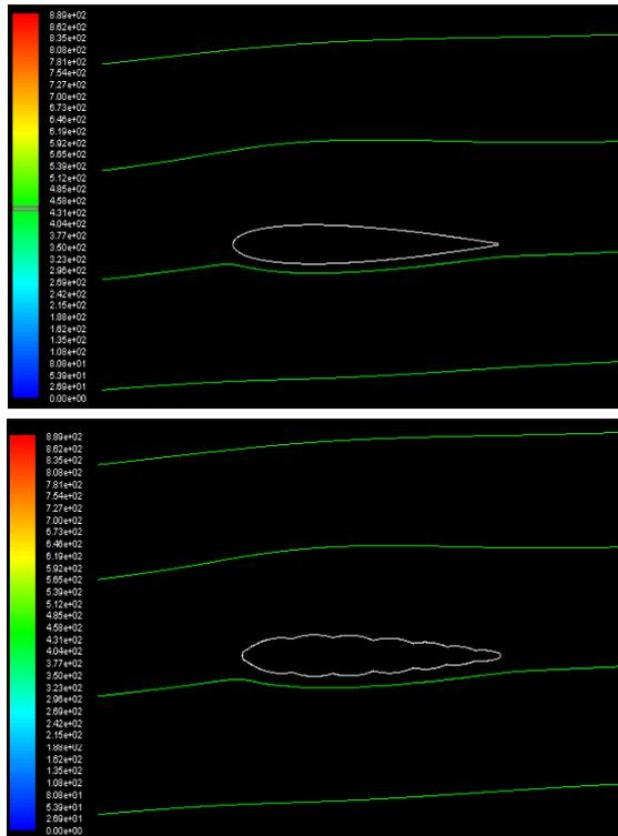
Fig. 10 streamline of NACA0012 and the inflatable wing
