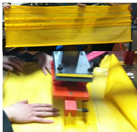
Fig. 16 heat sealing of the internal structure
