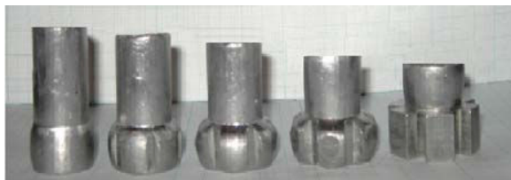
Fig. 14. Teeth formation stages for 3 and 6 teeth parts
