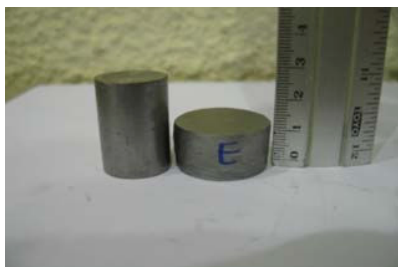
Fig. 2. Initial and final compressed lead specimen
