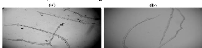
Fig. 1 Optical images (320x) of dispersed SWCNT (a) before, and (b) after the centrifugation step.
