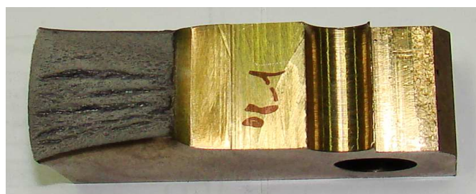
Fig. 19 CT sample after test without stable crack growth
