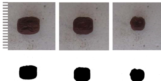
Fig. 5 Several steps of image analysis: Top row: original colour image of sample; Bottom row: image after thresholding (binary image)
