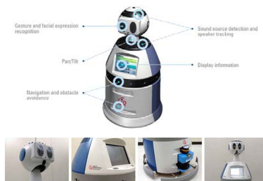
Fig. 1The Silvermate robot system
