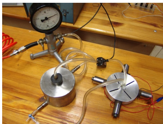
Fig. 20 The experimental setup for algae ultrasonication by system shown in Fig. 3b
