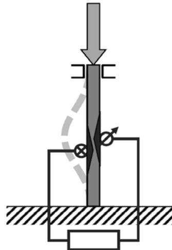
Fig. 2 Euler's column as an adaptronic system, cf. [12]
