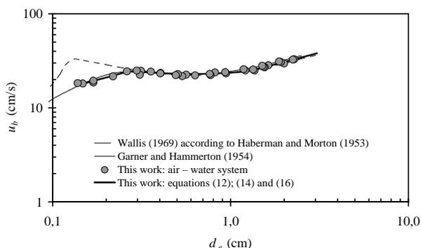
Fig. 6 Terminal velocity of air bubbles in air – water system
