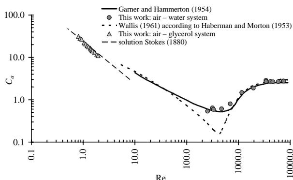
Fig. 5  $C_d$  versus Re
