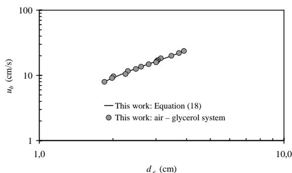
Fig. 7 Terminal velocity of air bubbles in air – glycerol system
