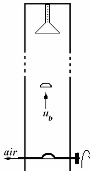
Fig. 1 Schematic of the experimental apparatus
