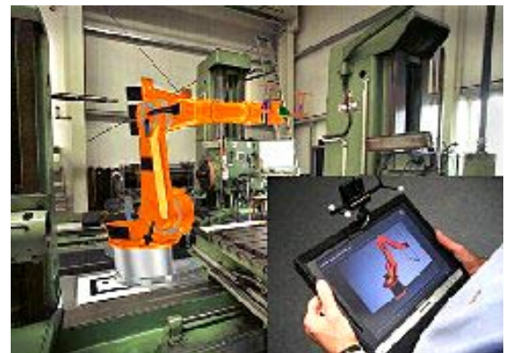
Fig. 4 Augmented Virtual Reality Manufacturing System
