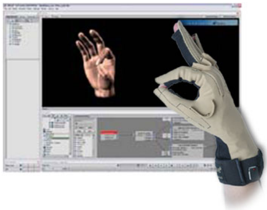
Fig. 2 Gloves with Sensors for Virtual Reality
