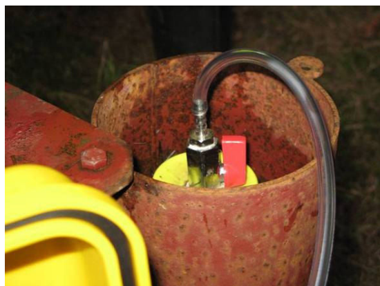
Fig. 2 A sample of landfill gas being pumped from a borehole well at the perimeter of an active landfill site
