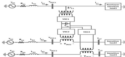
Fig. 2 Shunt and series compensators of GUPQC
