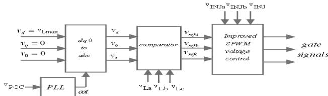
Fig. 5 Series compensator control
