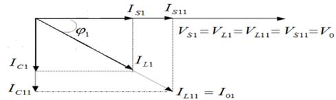
Fig. 6 Phasor representation of shunt compensator loading
