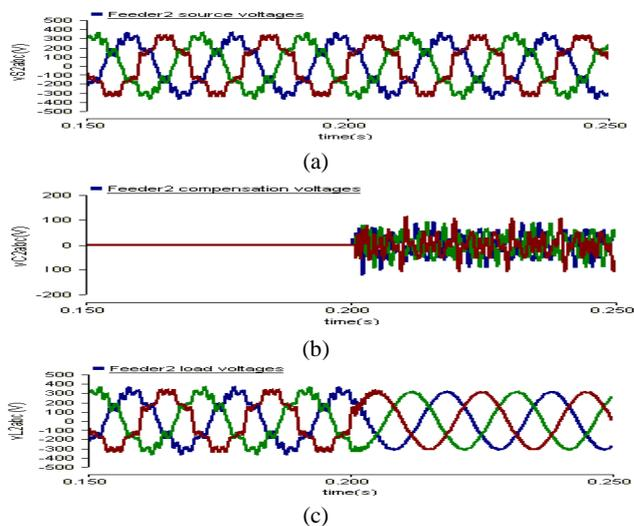
Fig. 13 Feeder2 voltages: (a) supply (b) compensation (c) load
