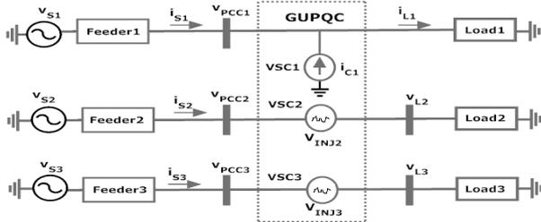
Fig. 1 Distribution system with the proposed GUPQC
