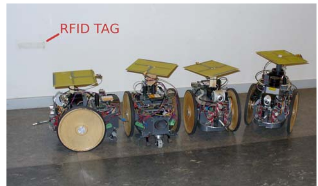
Fig. 5. Four MarsuBot robots used in the laboratory experiments. Directional RFID antenna on top of each robot. An RFID tag serving as a landmark can be seen on the background.
