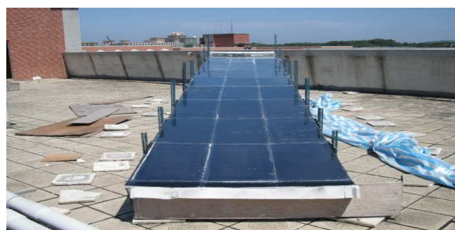
Fig. 12 Black-painted aluminum plate (Case 3)
