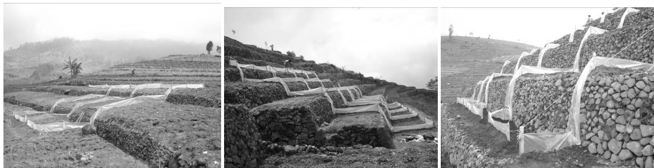
Fig. 3 Experiment plots in Pagersari village with stone terraces at slopes of 30% (left), 45% (center) and 75% (right)
