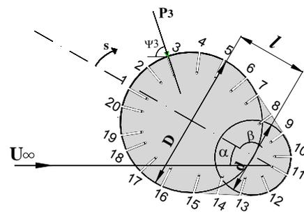
Fig. 2 Schematic diagram of a cam shaped tube
