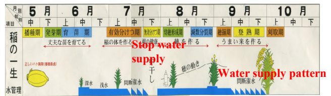
Fig. 24 Cropping pattern and water supply in paddy field
