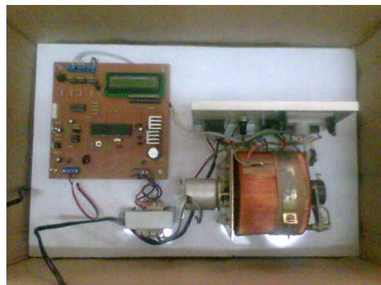
Fig. 9 A photo of constructed AVR system
