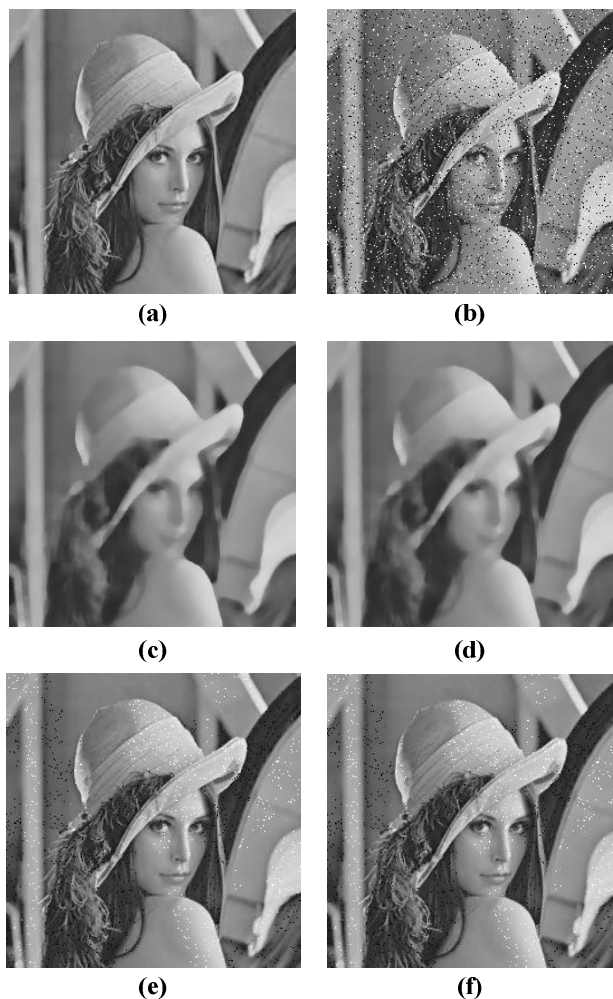
Fig. 1 Experimental Results on Lena's Picture; (a) the original image; (b) the noisy image corrupted by salt and pepper noise; (c) the outcome of Median filter; (d) the outcome of \alpha -trimmed mean filter; (e) the outcome of Median \epsilon -filter; (f) the outcome of \alpha -trimmed mean \epsilon -filter
