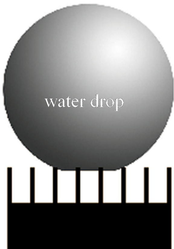
Fig. 1 Interaction of a water drop with structured surface according to the Cassie-Baxter model
