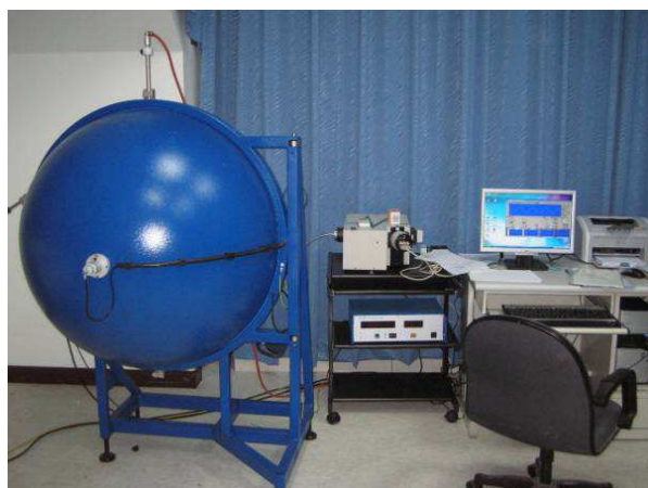
Fig. 2 Luminous flux measurement system
