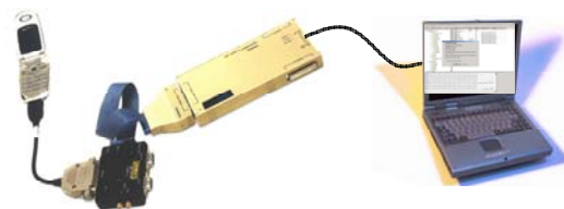
Fig. 2 Memory dump using JTAG
