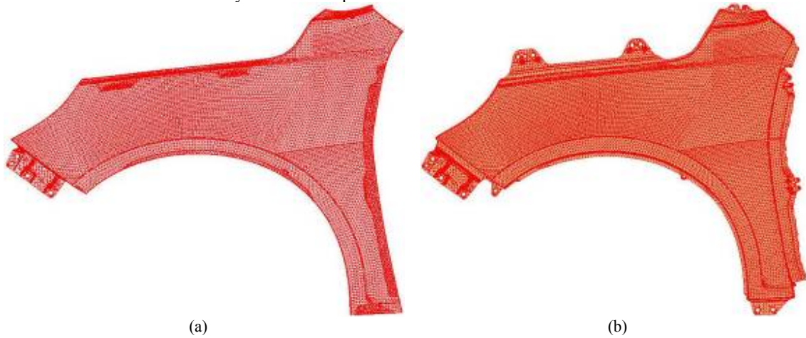
Fig.4 Flattening of fender (a) three dimensional surface, (b) flattening result
