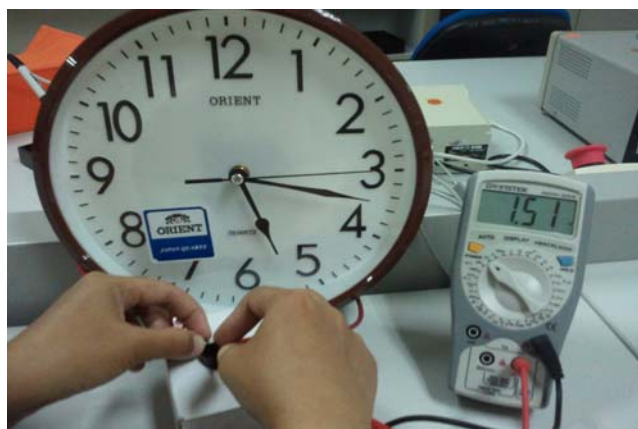
Fig. 6(a) One compacted vermicompost make wall clock's needle ticking
