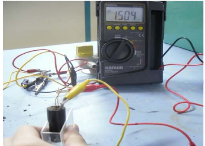
Fig. 2 One series of compacted vermicompost produces 1.504V
