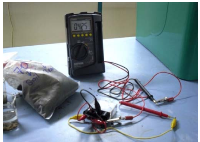
Fig. 3 Three series of compacted vermicompost produce 4.25V
