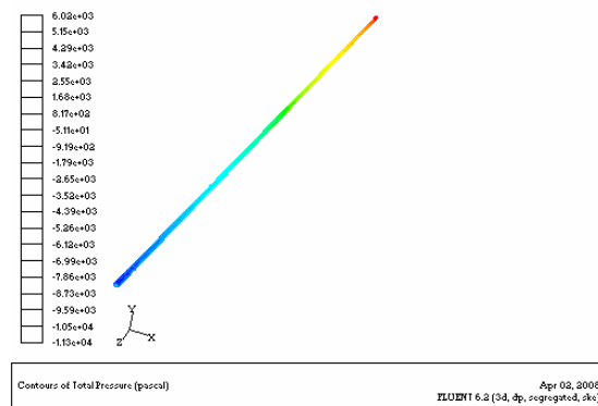
Fig. 3 Variation of total pressure for R134a at 40°C and G- 1058 kg/m 2 s at a quality of 0.5
