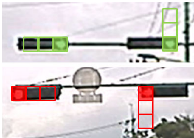
Fig. 8 Examples of traffic lights detection. Top picture is Prototypes of Haar-like feature for green traffic lights detection and down picture is Prototypes of Haar-like feature for red traffic lights detection
