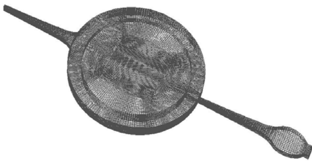
Fig. 2 The surface mesh distributions of present contoured nozzle/diffuser valveless micropump
