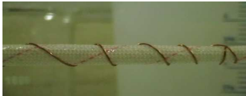
Fig. 1 Test section with insulation
