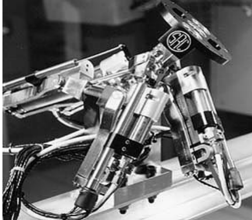
Fig.1.The hydraulic shoulder manipulator in movement
