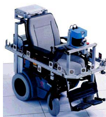
Fig. 11 MAid robot (from [26]) : typical example of a robotized wheelchair whose sensors and computer equipment make it similar in some extent to a mobile robot.
