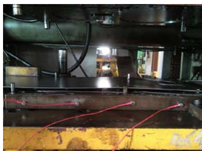
Fig. 10 Photograph set up a sensor to 150ton press (CH-1, 2, 3, 4 from the left side)
