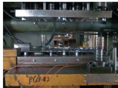
Fig. 13 Photograph set up a sensor to 150ton press (CH-1, 2, 3, 4 from the left side)
