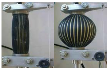
Fig. 2. Photograph of deflated and inflated state of the PPAM
