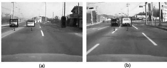
Fig. 12 Distinction of vehicle position. (a) Vehicle detection of both directions. (b) Vehicle detection of same direction.
