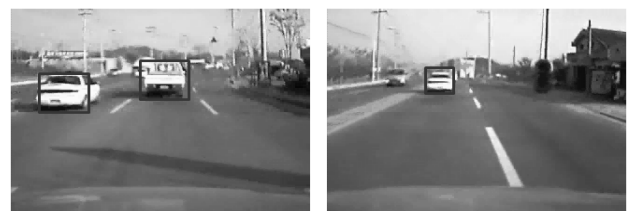
Fig. 10 Same directional vehicle detection of using haar-like and adaboost.
