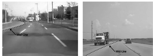
Fig. 6 Mid-line detection of road boundary.
