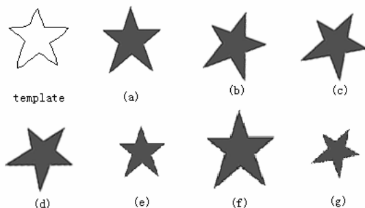
Figure.3 original template of a five-tips star and the matched images that are rotated or scaled up and down
