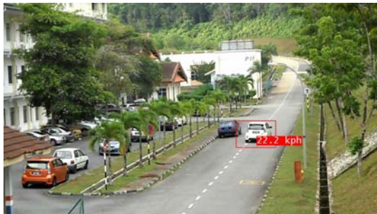
Fig. 3 Image sequence from upper left: (a) object shape extraction for centroid computation (b) centroid is pointed by red mark in ROI rectangular shape (c) speed computation as displayed in the image (d) continuous tracking with green box as current frame referred in previous images
