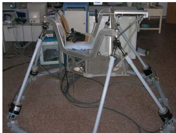
Fig. 1 The parallel motion platform with subsided cabin
