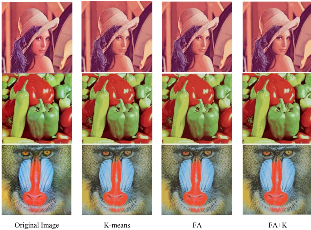
Fig. 5 Original image and quantized image in 16 colors from 3 methods; K-means, Firefly algorithm and our approach
