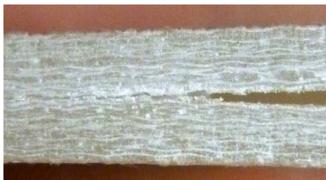
Fig. 6 Optical picture of the mid-section of an ECT tested specimen
